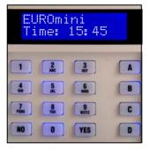
The manager menu is accessed by pressing 'D' and then keying in your **Manager** PIN code. The screen will display any relevant information; simply press '**No**' to move into Manager Menu.
